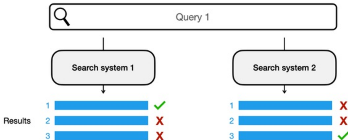
Figure 2-16. We need a scoring system that rewards system 1 for assigning a high position to a relevant result -- even though both systems retrieved only one relevant result in their top three results.
