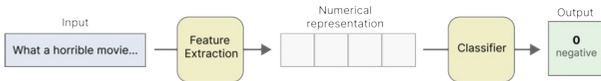
Figure 1-2. A common procedure for supervised text classification. We convert our textual input data to numerical representations through feature extraction. Then, a classifier is trained to predict labels.
