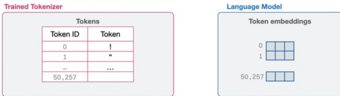
Figure 6-6. A language model holds an embedding vector associated with each token in its tokenizer.
