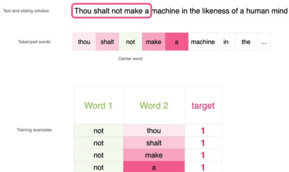
Figure 6-9. A sliding window is used to generate training examples for the word2vec algorithm to later predict if two words are neighbors or not.
