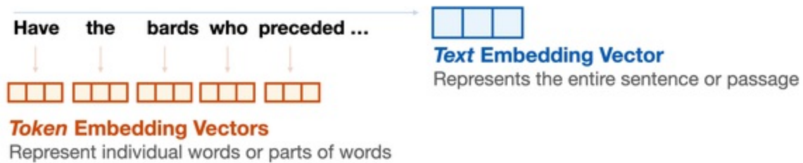
Figure 6-1. The difference between text embeddings (one vector for a sentence or paragraph) and token embeddings (one vector per word or token).
