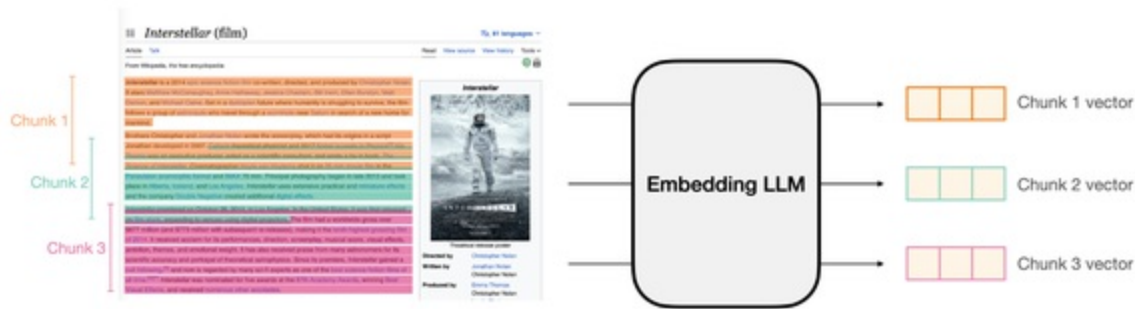
Figure 2-8. Chunking the text into overlapping segments is one strategy to retain more of the context around different segments.
