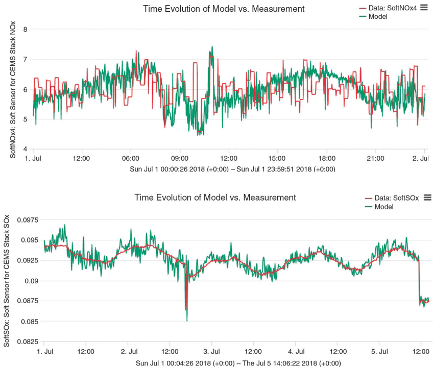
FIGURE 10.5 The computed value (dark gray) (green in web version) and the measured value (light gray) (red in web version) for NO x and SO x .
